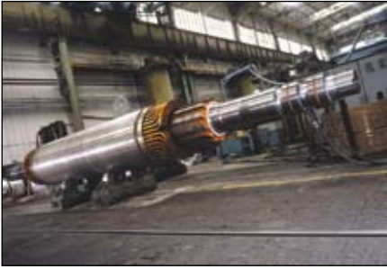
Rotor of a 220MW generator.
