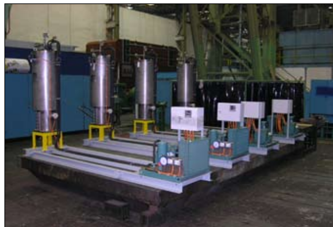
Compact hydrogen dryers delivered for 4 unit of NPP Dukovany, Czech Republic
