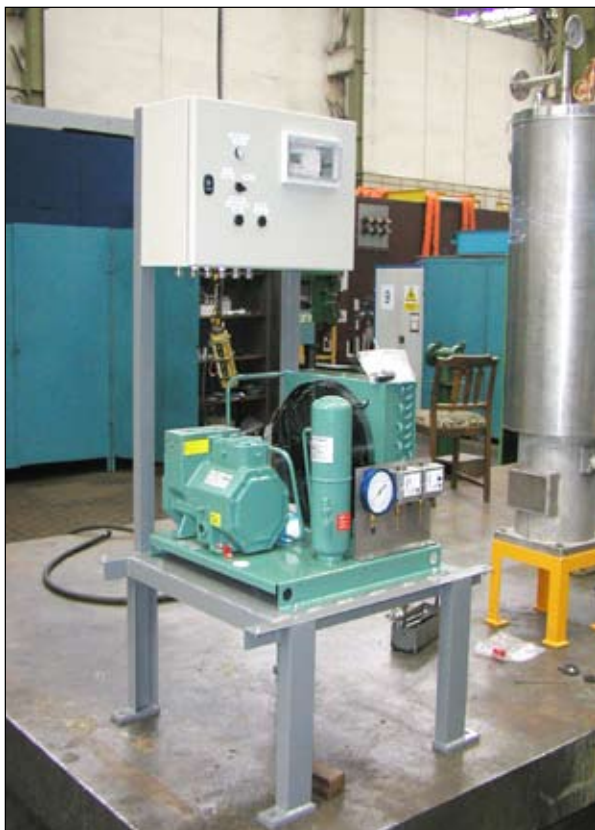
Condensation unit with control box
