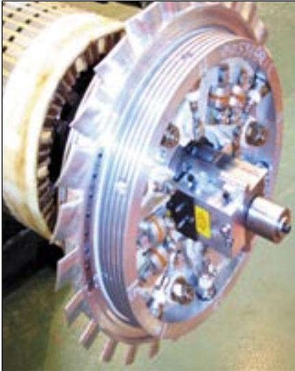
Fig.1 Transmitter fitted to generator rotor
