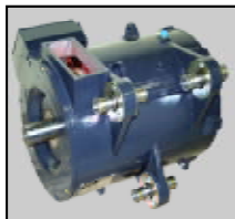
BLS motor for Swiss Railways. Force ventilated motor 213 kW.
