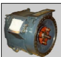
MDDM motor for Dutch Railways. Adtranz design. 334 kW.
