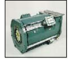
Double motor for Sprint Tram Amsterdam. Self ventilated motor 2 x 74 kW.
