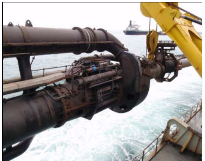
A BRUSH 4MW submersible motor with forced cooling fitted to the Gerardus Mercator vessel, supplied to Jan de Nul.
