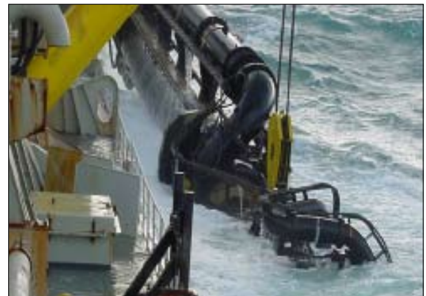
A BRUSH 4MW submersible motor assembled on the dredging arm, being lowered into position.
