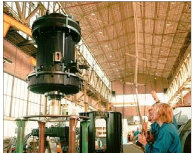
Final assembly of a new build submersible motor at our Ridderkerk facility
