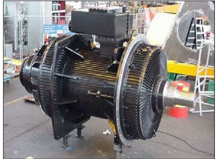
A BRUSH 2.6MW submersible motor with natural cooling arrangement supplied to Boskalis for the Prins der Nederlanden vessel.
