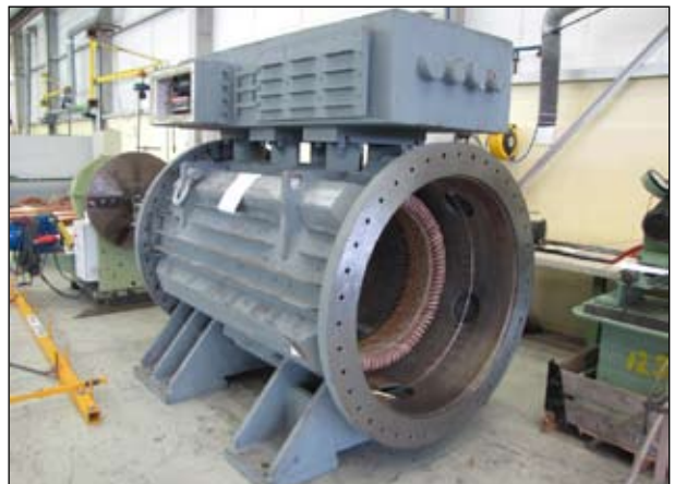
In works repair of a third party air cooled submersible motor.
