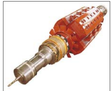
Completed rotor of a 30MW DG generator.
